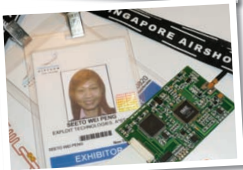
A typical RFID tag embedded in between a show pass. The UHF RFID reader module used was the size of a namecard, and saved hundreds of thousands of dollars in hardware costs!
